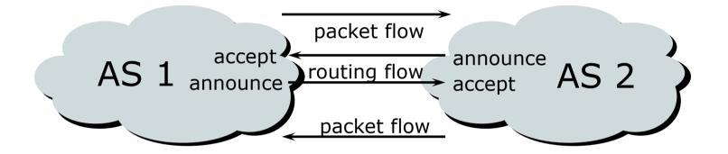
For networks in AS1 and AS2 to communicate: AS1 must announce to AS2 AS2 must accept from AS1 AS2 must announce to AS1 AS1 must accept from AS2
